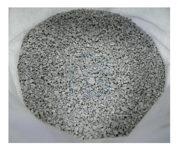
Silicon carbide molecules bonded together by the use of silicon nitride. The material is relatively low on corrosion and wears resistance compared to the sintered silicon carbide. But it scores in terms of economic application, where high performance is not a prerequisite. And is common in the case of metal alloy components.
